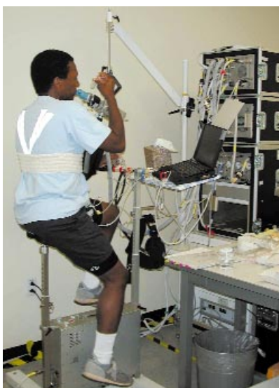
ARMS measurements are taken during exercise, with astronaut subject Mike Anderson, in a ground-based test of the equipment.
