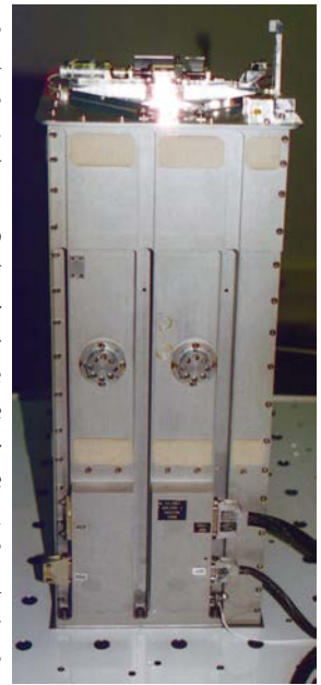
SOLCON-3 radiometer unit sitting atop FREESTAR. The digital processor unit is out of view to the right.
