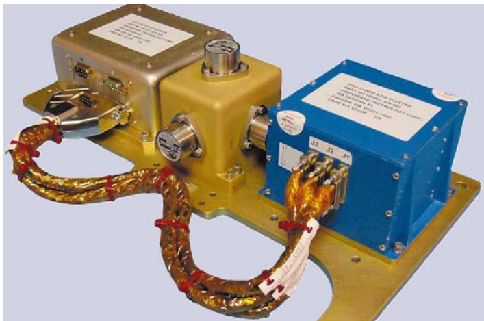
SAMS-FF includes the control data unit (left), a triaxial sensor head (center) and the fiber-optic gyroscope (right). Two additional triaxial sensor heads will be remotely mounted with payloads.
